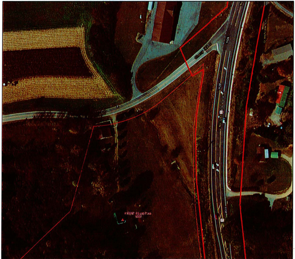
Area of Potential Effects outlined in red at location of Cherry Farm. Extends 75' from the centerline each way and 125' at the intersection of each road.
